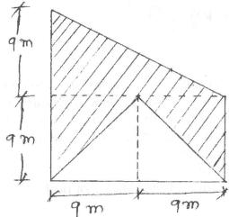
(b) Figure shows acceleration-time diagram for rectilinear motion. Construct velocitytime and displacement-time diagrams for the motion assuming that the motion starts with initial velocity of 5 m/sec from starting point.
