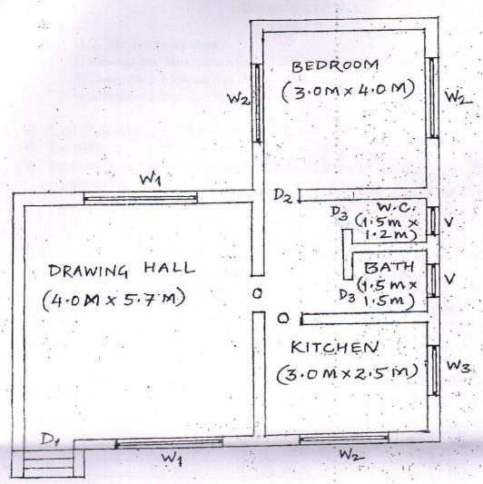
Wall Thickness - 300 mm. plinth level - 600mm. Floor to floor height - 3000 mm. Slab thickness - 120 mm.
