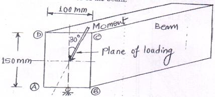
(C) Using moment area method, determine the vertical deflection and slope at 07 free end of the beam as shown in figure.
