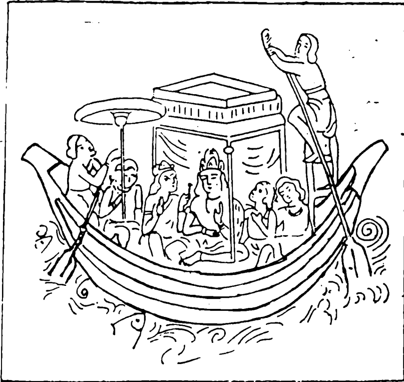
Fig. 5 : A pleasure-boat of Ajanta wall-painting used in shallow water and moved by a long paddle as steering oar and another short paddle to row and propel.
