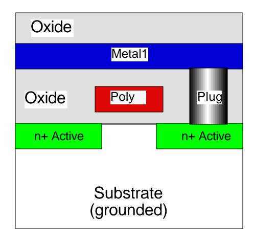
A contact or via is needed to connect two layers
