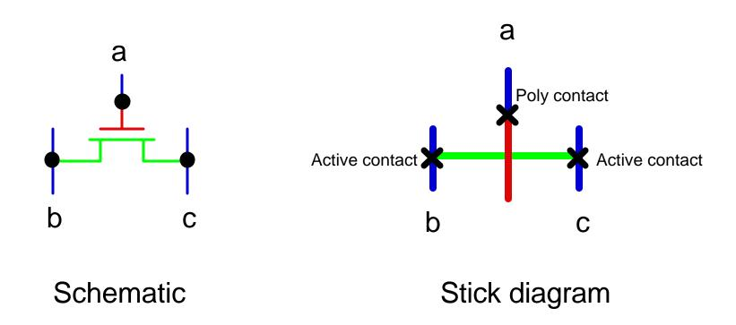
Poly contact: Metal1-to-Poly Active Contact: Metal1-to-Active
