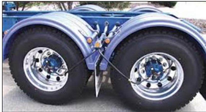
Figure 12 CTIS deployed on a trailer 1 CTIS deployed on a trailer
