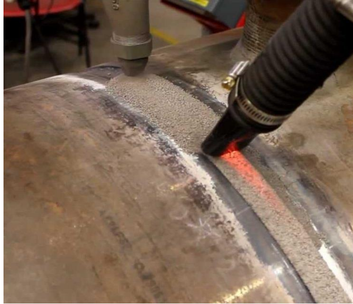
Figure 5.3 Submerged Arc Welding
