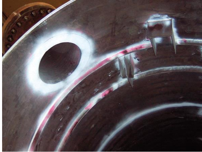
Figure 5.4 Die Penetration Test
