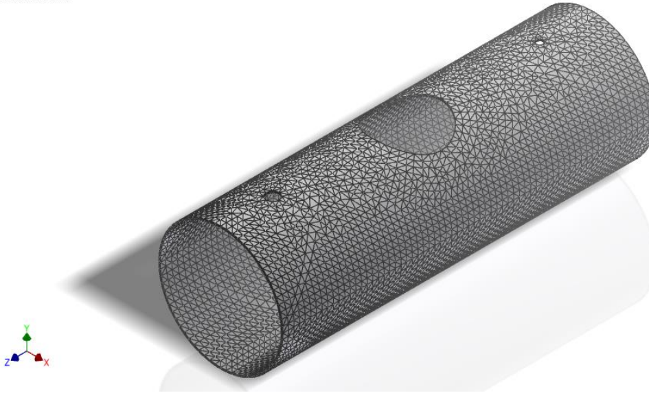
Figure 7.15 Mesh View of Shell
