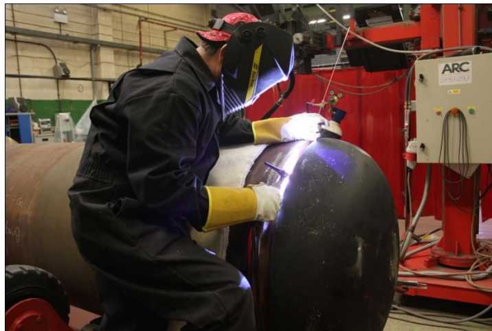
Figure 5.2 Manual Arc Welding
