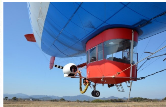
Figure 1.12 Closed Structure Gondola [13]
