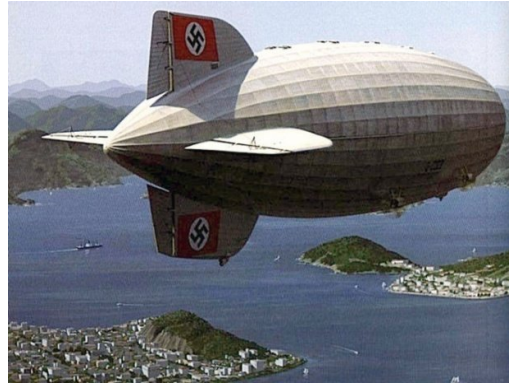
Figure 1.10 “+” type configuration of fin attachment [12]
