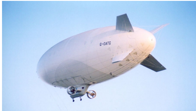
Figure 1.8 “X” type configuration for fin attachment [10]
