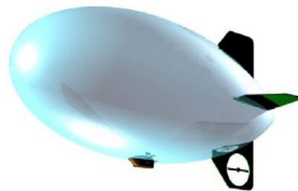
Figure 1.15 Airship with yaw motor mounted on fin [9]
