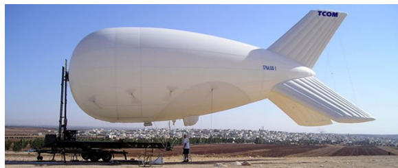
Figure 1.9 “Y” type configuration of fin attachment [11]
