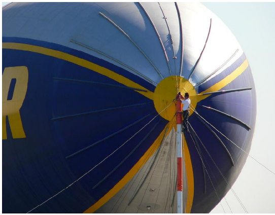
Figure 4.16 Nose Batten of an Airship [23] Fig 4.17 Deformed shape of bow stiffening [24]
