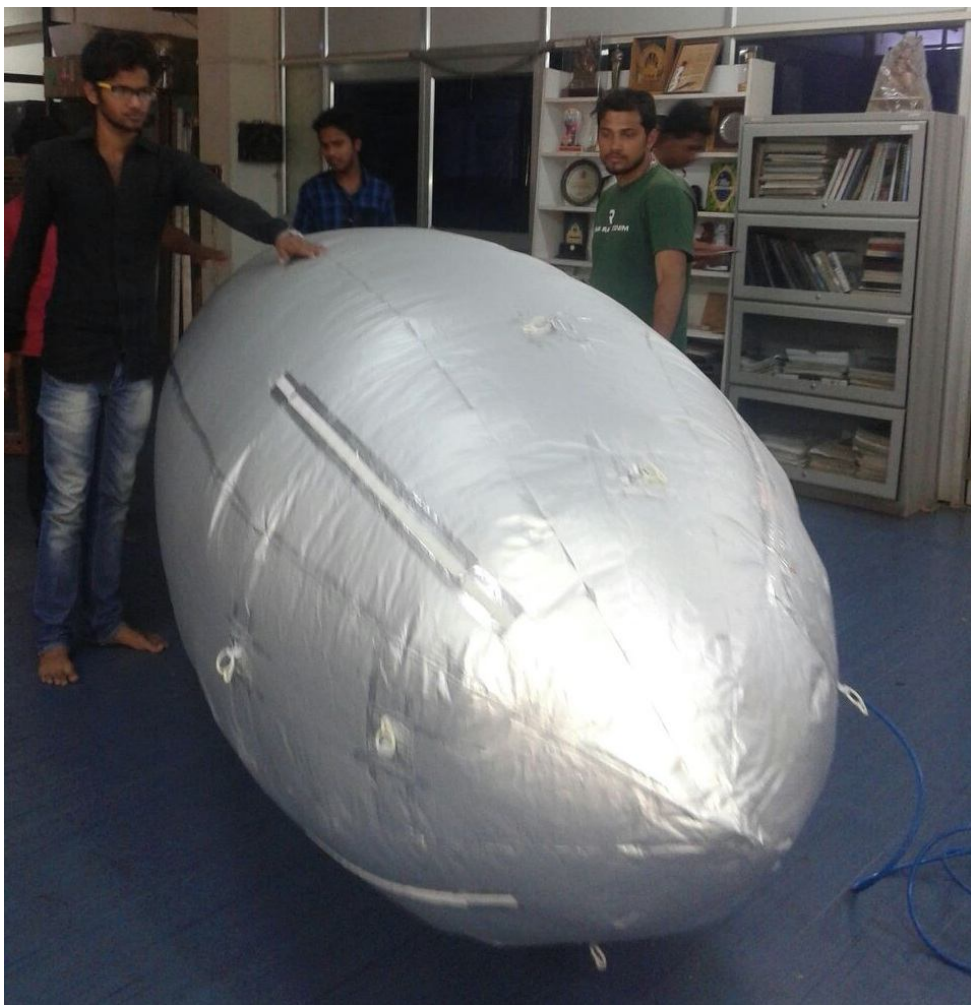
Figure: 5.13 final air filled envelope
