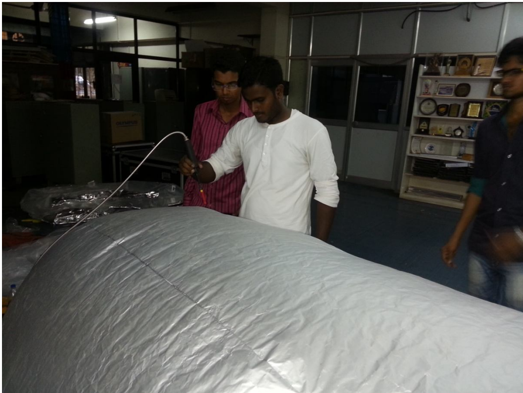
Figure 6.1 Leakage testing of envelope
