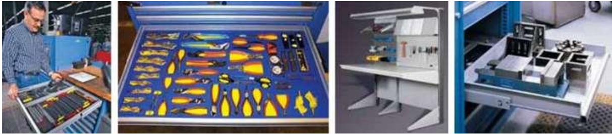
Fig 3.7- The 5S visual workplace, where tools are easy to find and located right at the working area, leads to a clean, efficient work environment.
