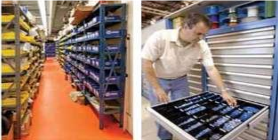
Fig 3.4- Open shelving (left) is very inefficient at storing small items. High density drawer and shelf storage (right) enables storage of small items in right-sized compartments, increasing cubic capacity and organization.
