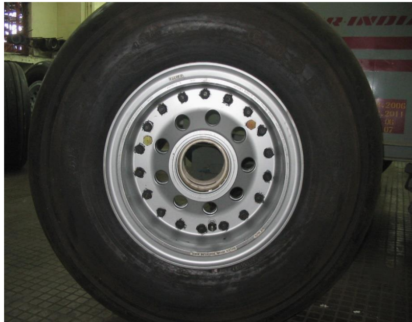
Figure 5.Complete assembly of Main Wheel
