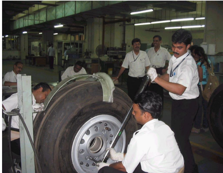
Figure 4.Final Torqueing to Nuts
