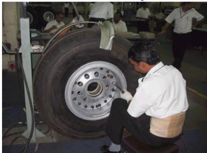
Figure 3. Tightening the Nuts with a Hydraulic Torque Wrench
