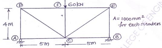
(ii) Using Unit Load Method or Castigliano's second theorem, for rigid jointed 08 frame as shown in fig. Find horizontal displacement of roller support.
