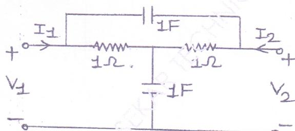
(b) For the network, calculate  $i_1$ ,  $i_2$ ,  $\frac{di_1}{dt}$ ,  $\frac{di_2}{dt}$ ,  $\frac{d^2i_1}{dt^2}$ ,  $\frac{d^2i_2}{dt^2}$  at  $t=0^+$ . Switch is closed at  $t = 0$ . Initially switch is open.
