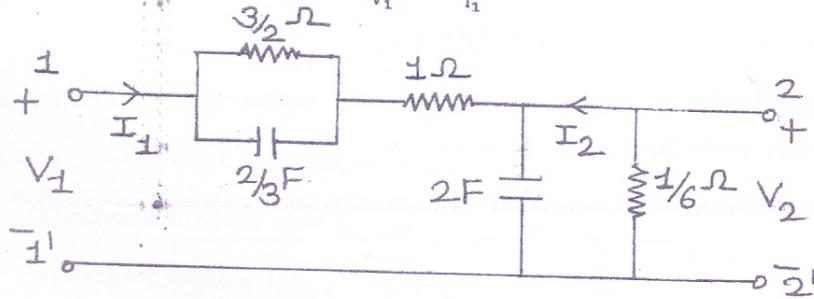
5.(a) For the given network at  $t = 0$ , switch is opened. Calculate  $v$ ,  $\frac{dv}{dt}$ ,  $\frac{d^2v}{dt^2}$  at  $t=0^+$ .
