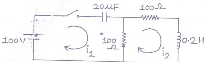
7. (a) Find the driving admittance  $Y(s)$  for the network shown below and plot the pole zero diagram. 10
