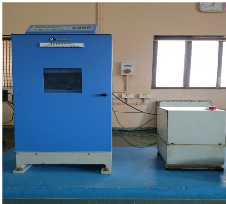
Fig 4.1: Compression Testing Machine (3000 KN Capacity)
