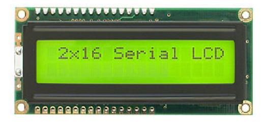
Various display device such as seven segment display. LCD display, etc can be interfaced with microcontroller to read the output directly. In our project we use a two line LCD display with 16 characters each.Liquid crystal Display (LCD) displays temperature of the measured element, which is calculated by the microcontroller. CMOS technology makes the device ideal for application in hand held, portable and other battery instruction with low power consumption.
