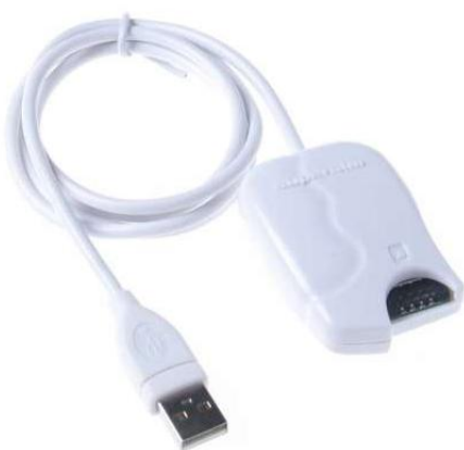
Fig-3. Simcard Cloning hardware device
