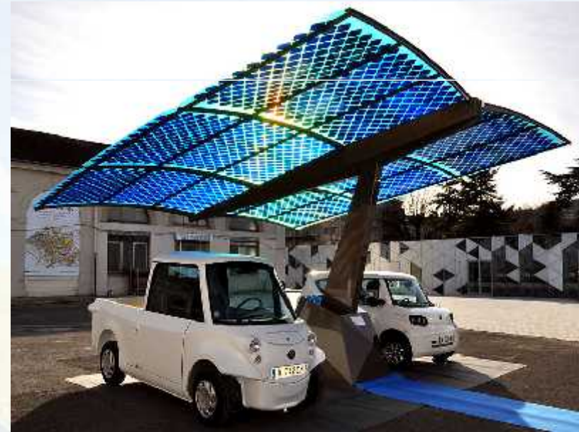
A mobile station that replenishes energy for electric vehicles using solar energy.
