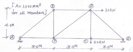
6. (a) Using Virtual Work Method, for rigid jointed frame as shown in fig. Find 10 horizontal displacement of roller support. Take EI = Constant.
