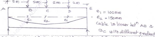
Estimate short term deflection due to Initial Prestressing force, Self weight of beam and Imposed load. Also estimate long time deflection considering Ec of concrete reduces to 2/3 of its initial value and n=0.8. Compare deflections with permissible limits. [15]
