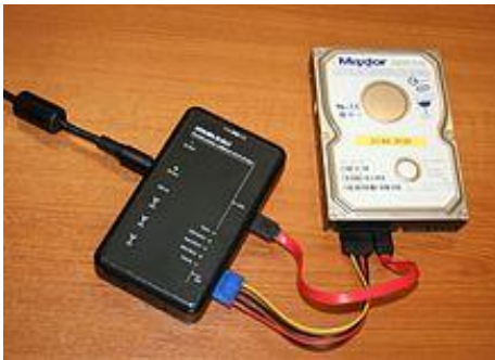
Figure 2.7(b) HDD write block device
