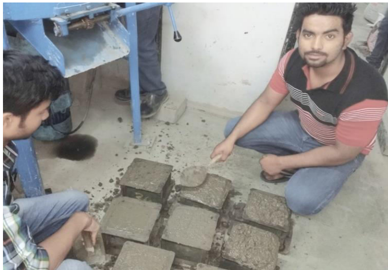
Fig:3.4: Placing of Concrete.
