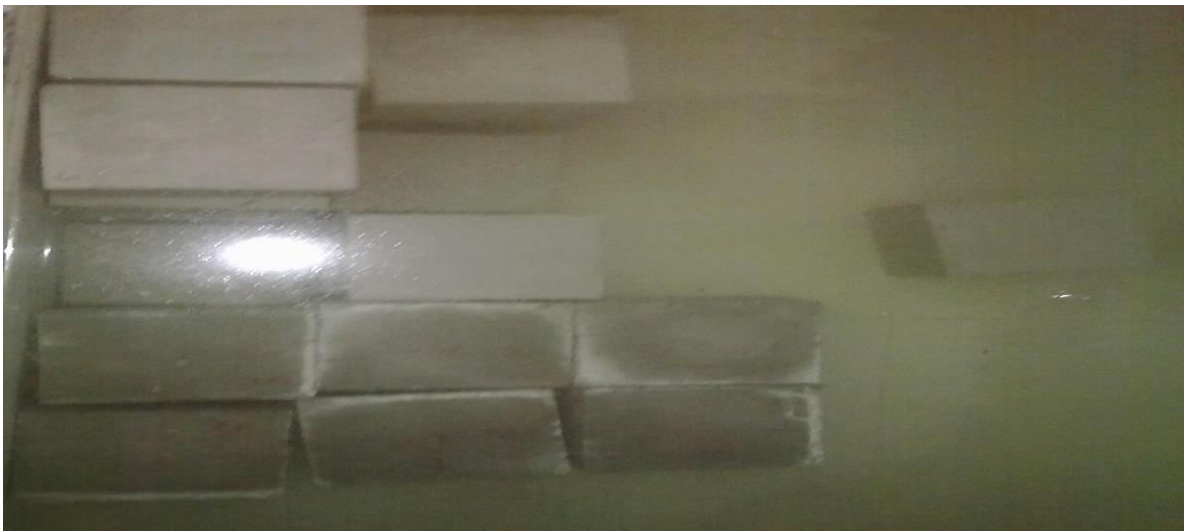
Fig: 3.7. Curing of Concrete
