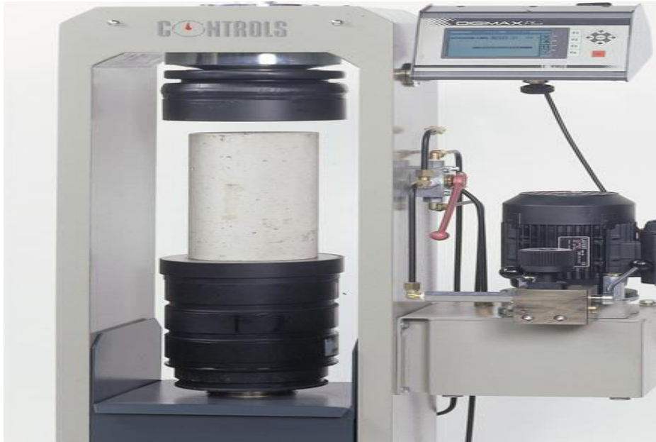
Fig: 3.12: Compressive Strength Testing Machine
