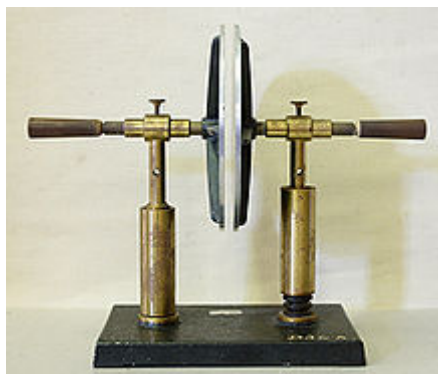
A simple demonstration of a parallel-plate capacitor
