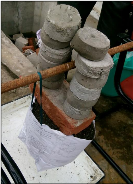
Fig.4.6.4.Static Load Capacity Testing
