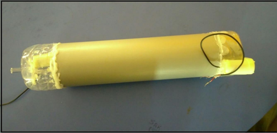
5. Ballast tank with two pump
