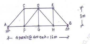
Find the vertical deflection of the truss shown in figure at the joint C. Cross-sectional areas in mm<sup>2</sup> of all the members are shown in figure. Take  $E = 2 \times 10^5$  N/mm<sup>2</sup>.
