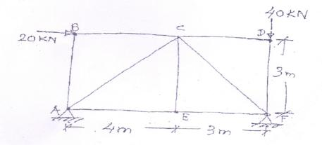
4. Analyse the frame using Stiffness method. Draw BMD.
