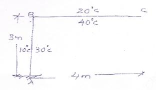
2. Analyse the frame using flexibility method and draw BMD
