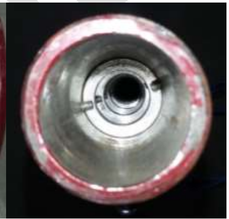
Fig.9. Insert blockage in pipe.
