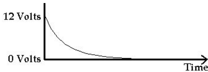
Figure 3.9: Voltage vs time curve during discharging
