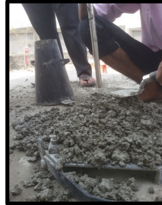
Fig. 4.3 Slump Cone Test
