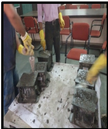
Fig. 4.4 Flling of Cube Mould
