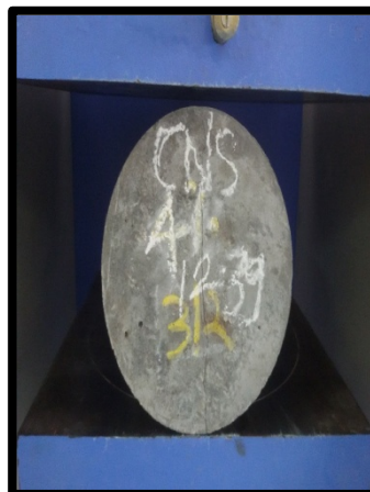
Fig. 4.10 Testing of Cylindrical Sample
