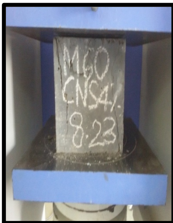
Fig. 4.9 Testing of Cube Sample
