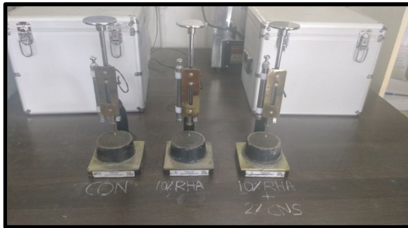
Fig. 6.1 Arrangement for Vicat Test
