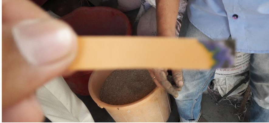
Fig 9: Litmus paper indicating the pH value of Concrete.
