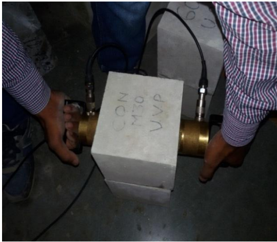
Fig 17: Test of bacterial concrete samples using Ultrasonic Pulse Velocity Machine.
