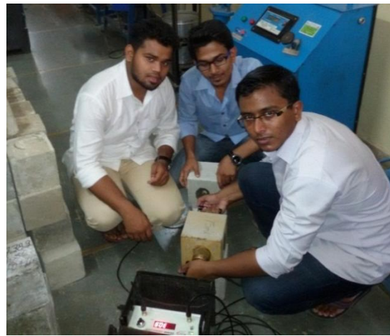
Fig 17: Test of bacterial concrete samples using Ultrasonic Pulse Velocity Machine.
