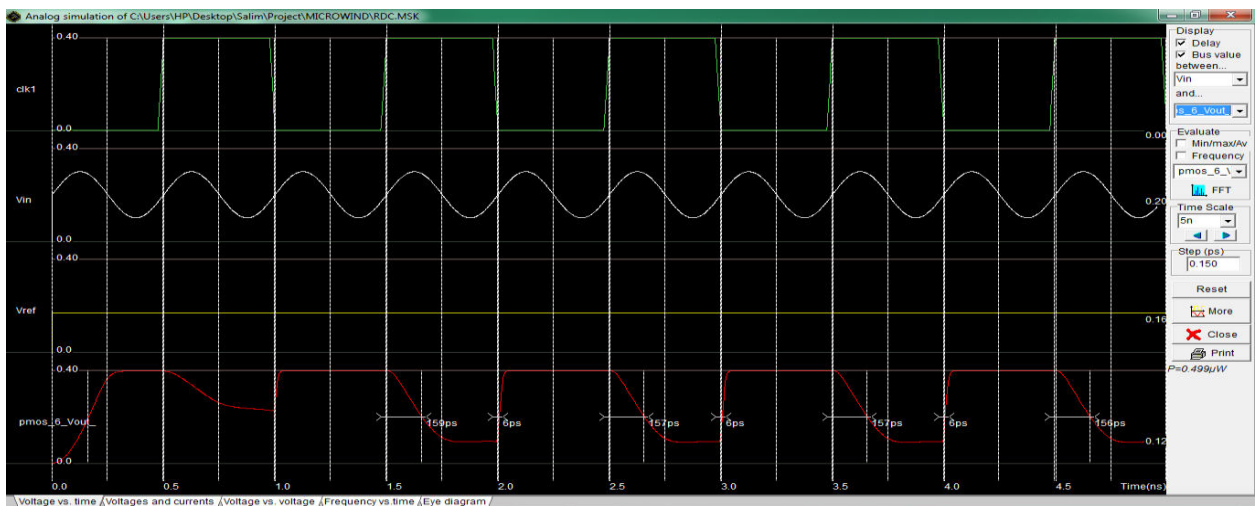
Fig.8.13 Simulation of RDC using CMOS 45nm
