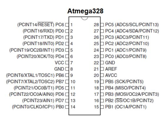
Each of the 14 digital pins on the Uno can be used as an input or output, using pinMode(), digitalWrite() and digitalRead() functions. They operate at 5 volts. Each pin can provide or receive 20 mA as recommended operating condition and has an internal pull-up resistor (disconnected by default) of 20-50k ohm. A maximum of 40mA is the value that must not be exceeded on any I/O pin to avoid permanent damage to the microcontroller.
