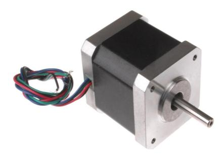
DC brushed motors rotate continuously when DC voltage is applied to their terminals. The stepper motor is known by its property to convert a train of input pulses (typically square wave pulses) into a precisely defined increment in the shaft position. Each pulse moves the shaft through a fixed angle.
