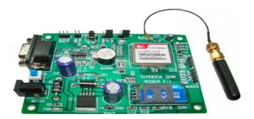
In addition, the GSM900 device integrates an analog interface, an A/D converter, an RTC, an SPI bus, an I<sup>2</sup>C, and a PWM module. The radio section is GSM phase 2/2+ compatible and is either class 4 (2 W) at 850/ 900 MHz or class 1 (1 W) at 1800/1900 MHz.
