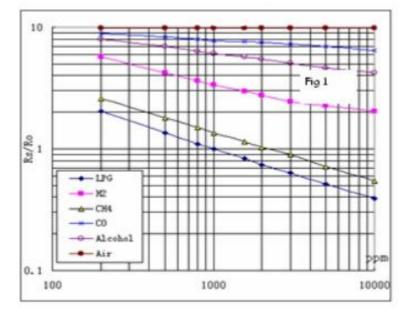
Fig. shows the typical sensitivity characteristics of the MQ-6, ordinate means resistance ratio of the sensor (Rs/Ro), abscissa is concentration of gases. Rs means resistance in different gases, Ro means resistance of sensor in 1000ppm LPG. All test are under standard test conditions.
