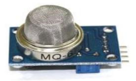
Sensitive material of MQ-6 gas sensor is SnO<sub>2</sub>, which with lower conductivity in clean air. When the target combustible gas exist, the sensor's conductivity is more higher along with the gas concentration rising. Please use simple electrocircuit, Convert change of conductivity to correspond output signal of gas concentration.
