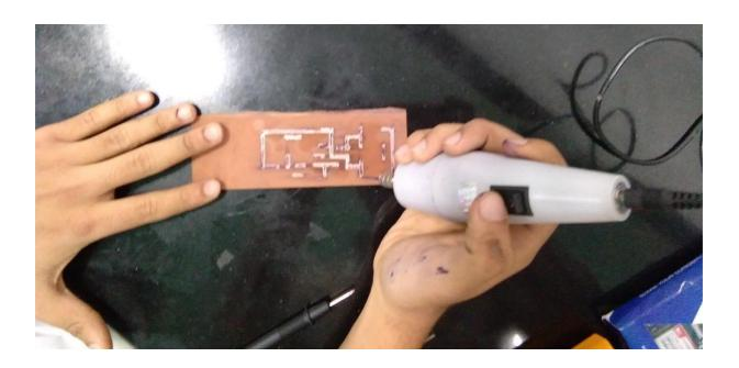
The Printed Circuit Board is now ready for mounting the components on it.
