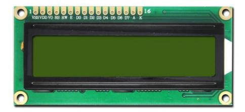
The command register stores the command instructions given to the LCD. A command is an instruction given to LCD to do a predefined task like initializing it, clearing its screen, setting the cursor position, controlling display etc. The data register stores the data to be displayed on the LCD. The data is the ASCII value of the character to be displayed on the LCD. Click to learn more about internal structure of a LCD.
