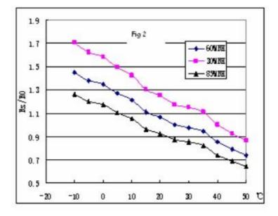
Fig. shows the typical temperature and humidity characteristics. Ordinate means resistance ratio of the sensor (Rs/Ro), Rs means resistance of sensor in 1000ppm Methane under different tem. and humidity. Ro means resistance of the sensor in environment of test conditions. 1000ppm Propane, 20°C/65%RH
