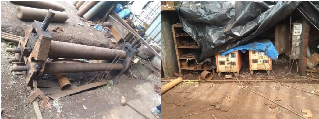
Fig. 4.3. POOR PLACEMENT OF MACHINING EQUIPMENT.
