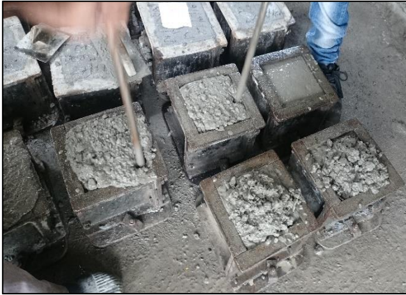
Figure 4.1 Filling the cube moulds
