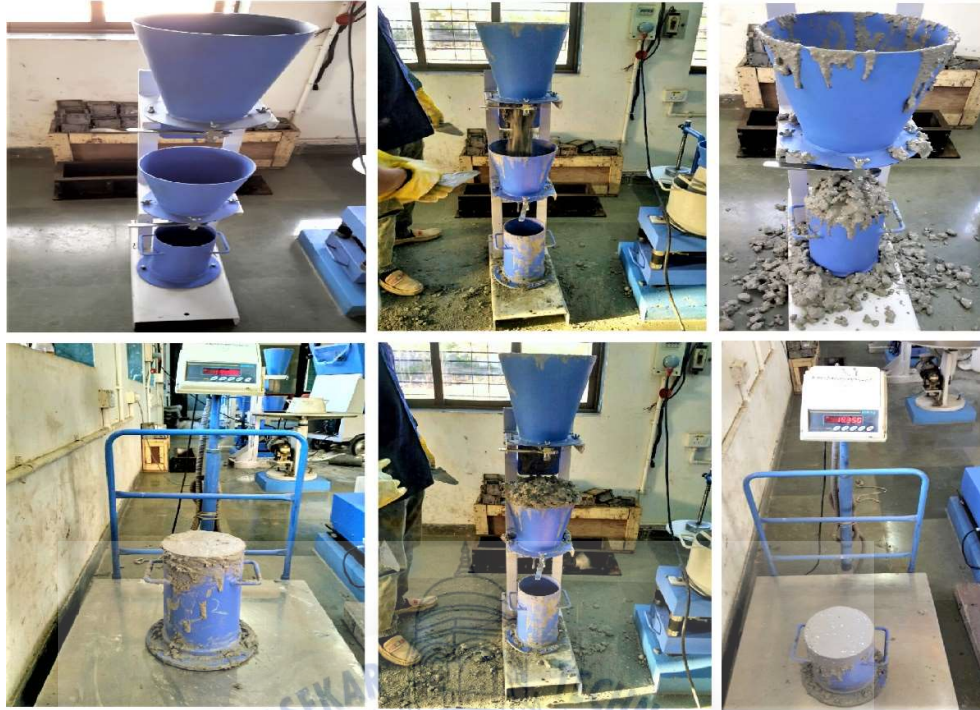
FIG 5.11: COMPACTION FACTOR TEST
