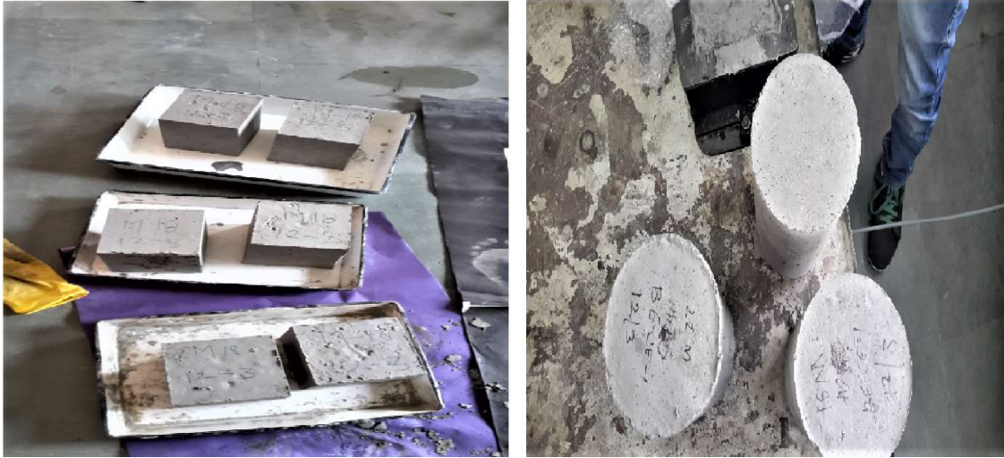
FIG 5.16: DEMOULDED GEOPOLYMER CONCRETE SPECIMENS
