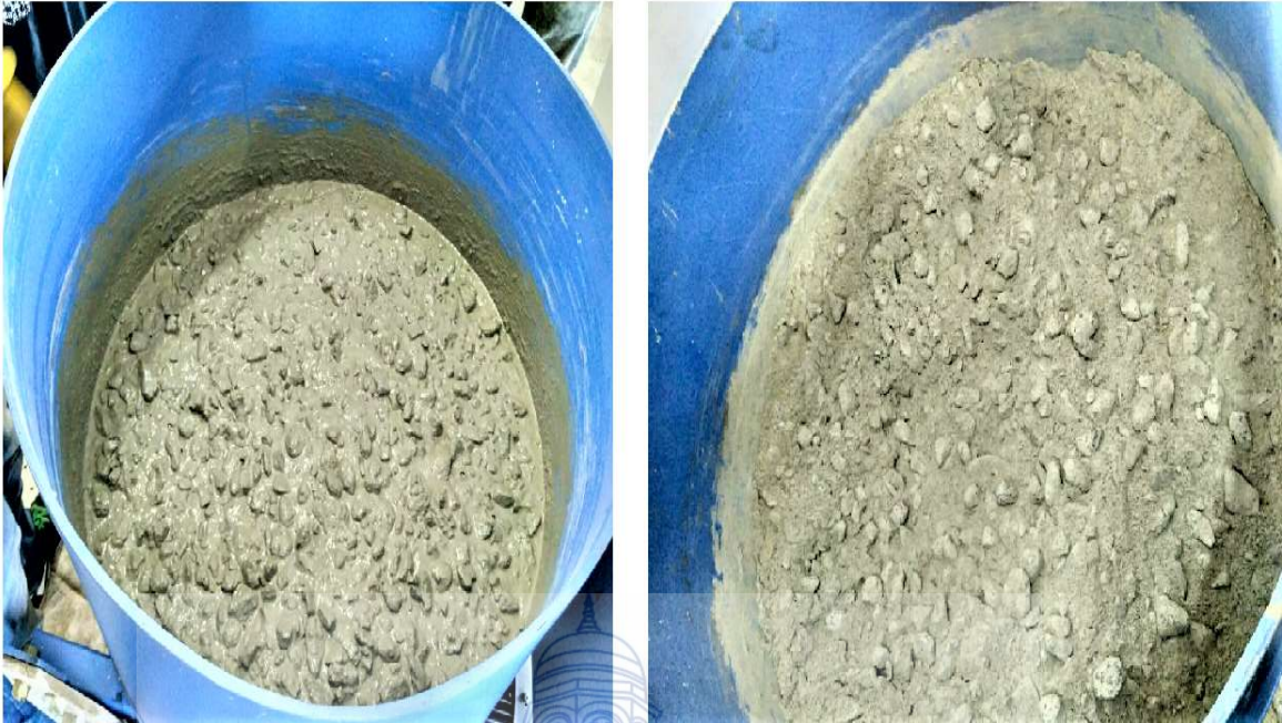
FIG 5.7: WET AND DRY MIX OF CONCRETE IN MIXER (PAN STATIONARY)
