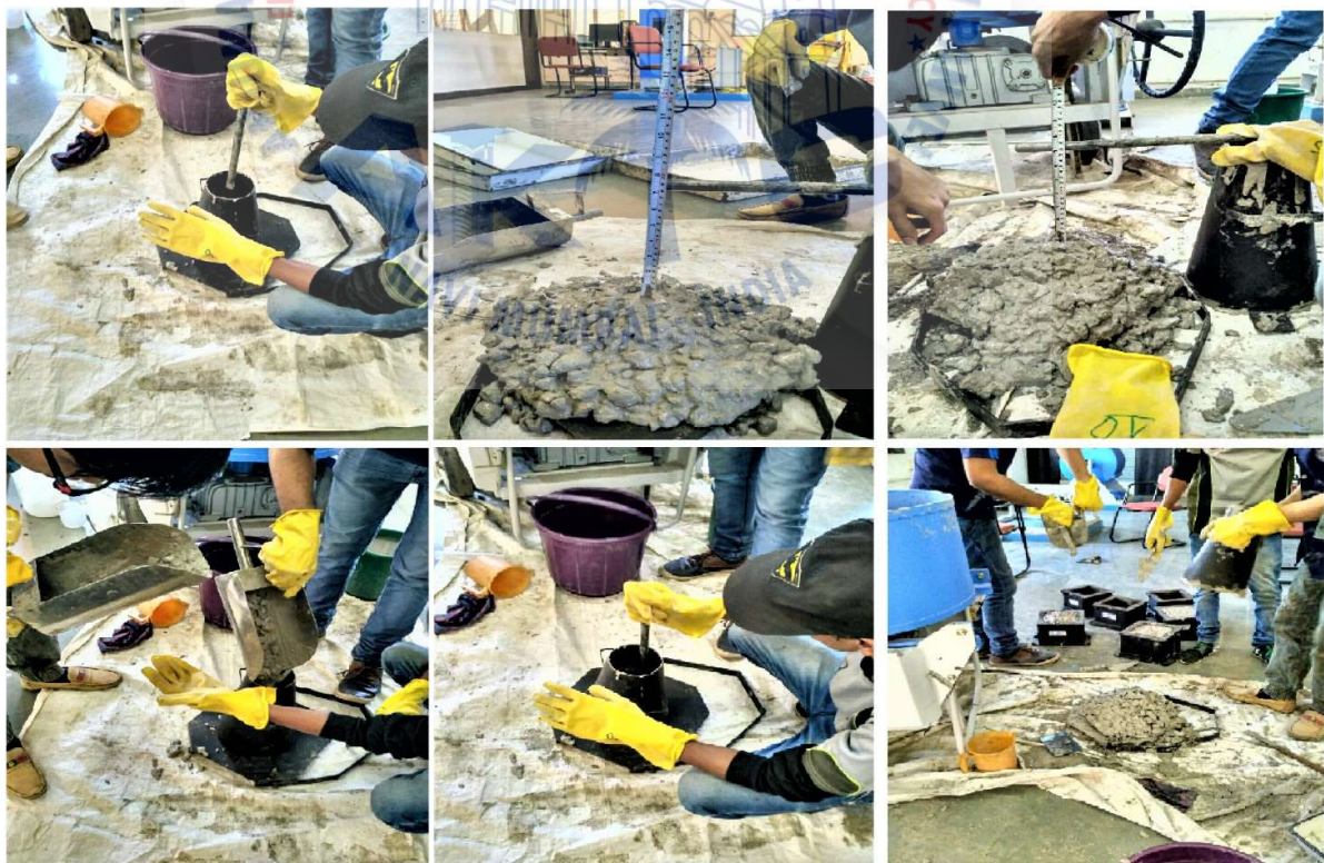
FIG 5.10: SLUMP CONE TESTING ON FRESH CONCRETE
