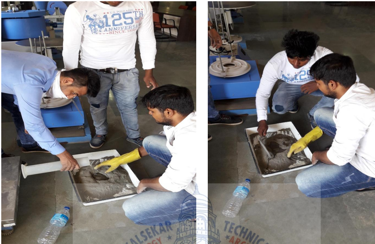
Fig 6: Mixing of cement mortar
