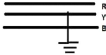
Figure 5: double line-to-ground fault
