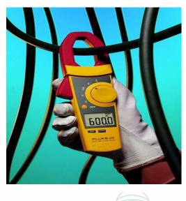
An electrical meter with integral AC current clamp is known as a clamp meter, clamp-on ammeter or tong tester.
