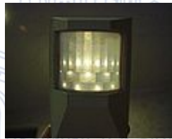
Fig 6.2 PID front cover only with point light source behind to show individual lenses.
