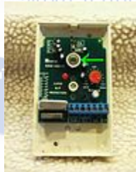
Fig 6.3 PID with front cover removed showing location of pyroelectric sensor.
