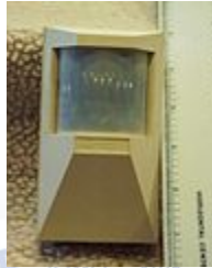
Fig 6. Typical residential and/or commercial PID with multi-Fresnel lens cover
