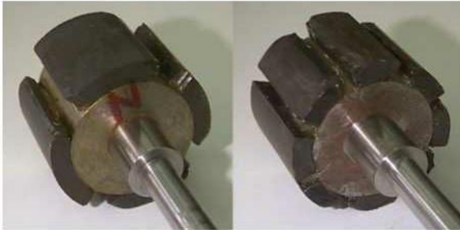
Fig5.2:- 4 pole and 8 pole –Permanent magnet rotor
