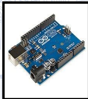
Figure 6.1: ARDUINO UNO SMD R3
