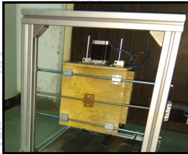
Figure 3.4: Y Axis lead screw of the machine
