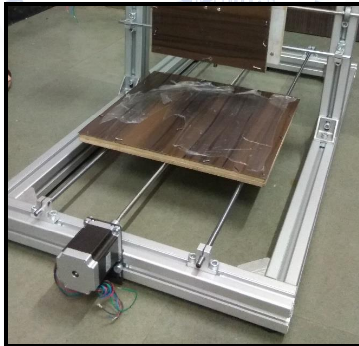
Figure 7.7: The bed, x-axis leadscrew and guide ways
