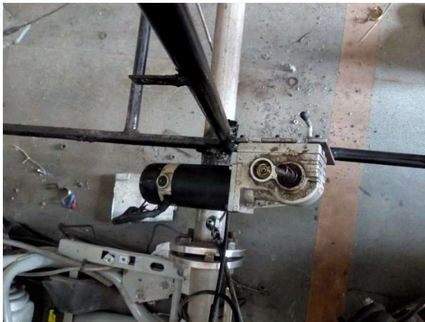
Figure 10.5. mounting of motor for controlling of steering
