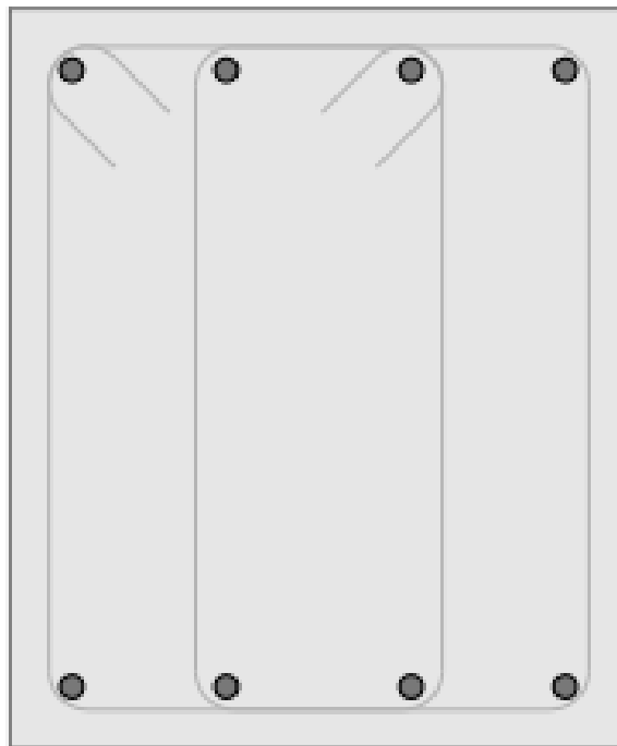
Figure 4.2 Beam section B
