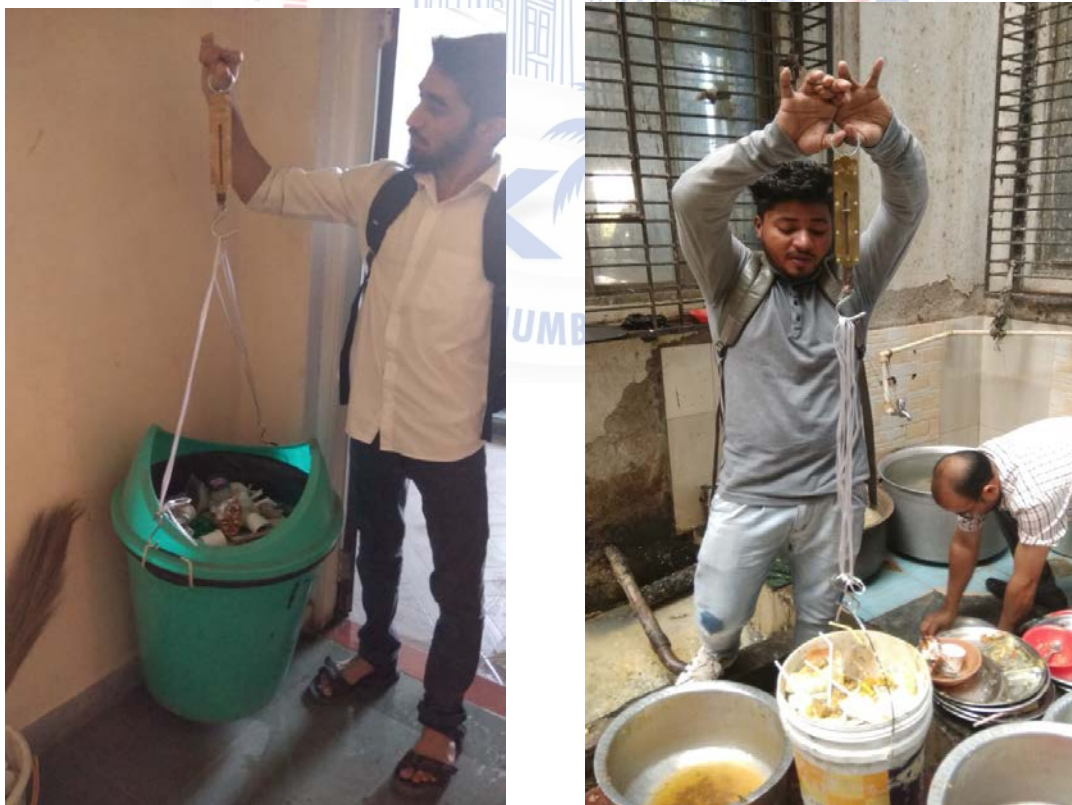
Figure 3.6 Calculating the weight of waste of different bins by using weighing balance
