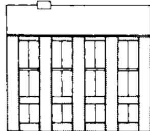
11-14 The perception of scale is changed by the ratio of the window area to the remaining area of wall as well as by architectural articulation (i.e. vertical, horizontal or mixed → 10); glazing bars can contribute substantially to this
