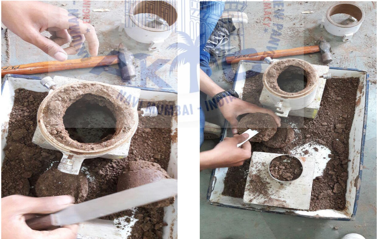
Fig 4.7 Performing Standard Proctor Compaction Test.
