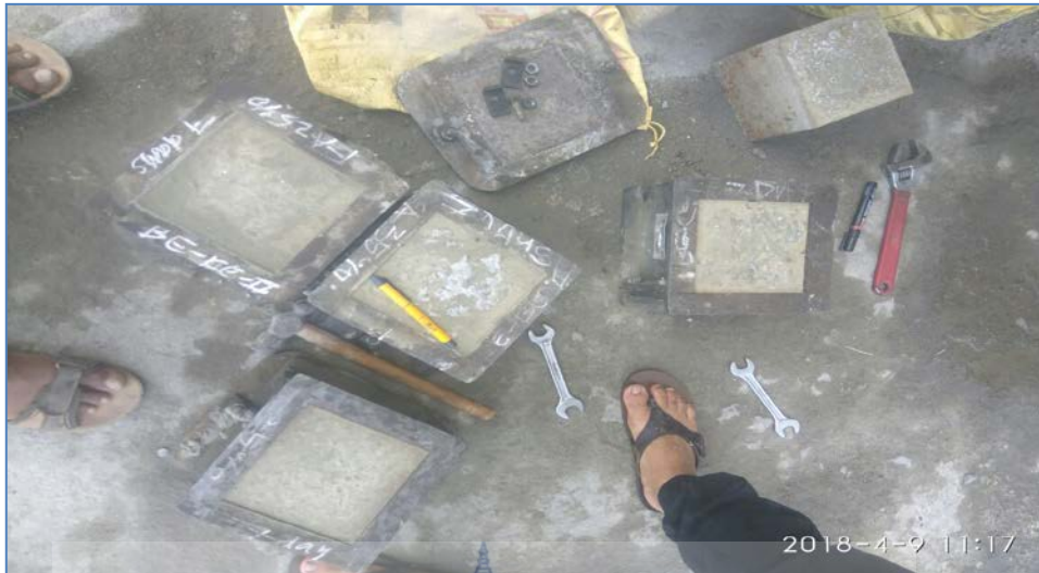
Figure 3.1 Preparation for the cube for normal curing
