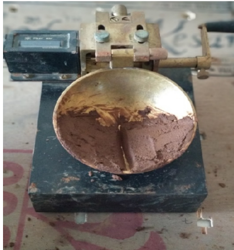
Figure 4.2.3 Casagrande's Apparatus and Soil Specimen in it
