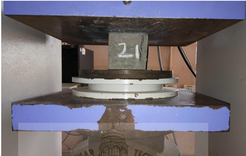
Fig 5.2: Compressive Strength Testing
