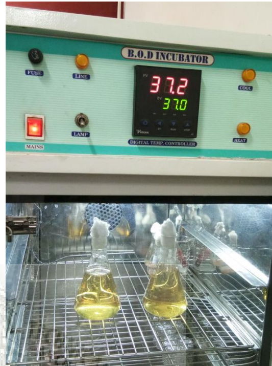
Fig 3.4: Placing the solutions in Incubator at 37°C
