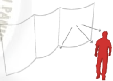
Figure 67 Reflection of Sound on Convex Walls
